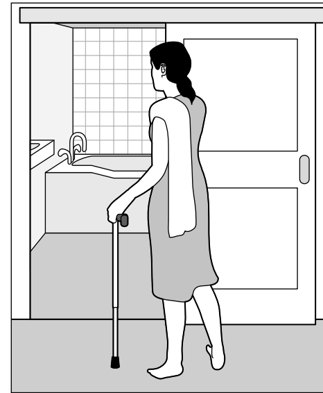
Install sliding doors if possible
