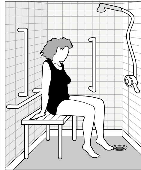
A wooden bench and grab-rails
