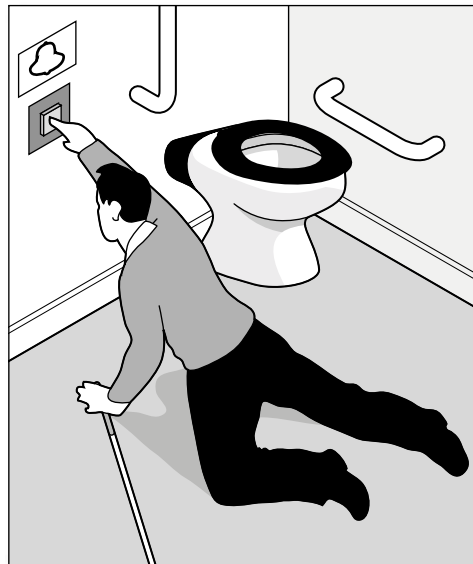
Ensure help alarm is accessible
